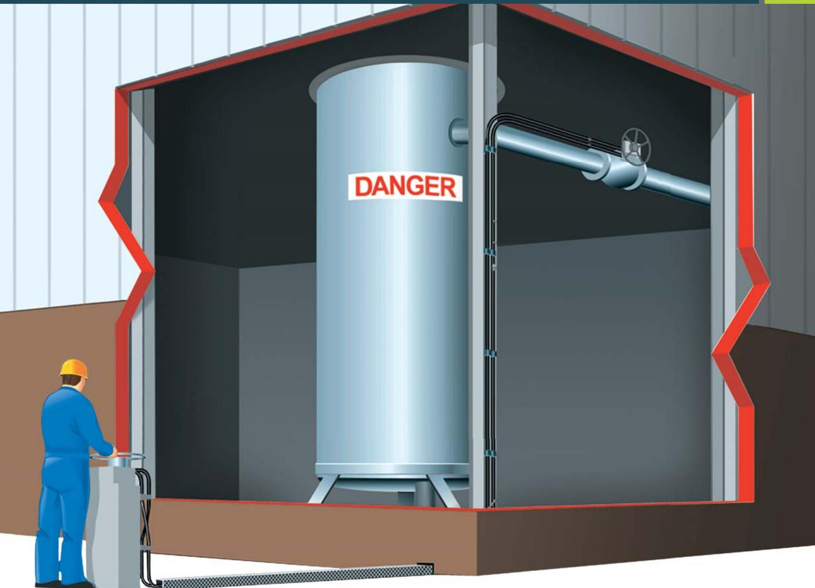
The cable system can be passed through walls, bulkheads, floors and any other obstacles to reach the valve.
